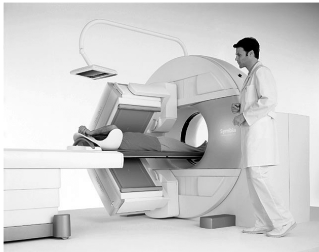
Figure 13 A scanner used for combined SPECT and CT imaging. The two rectangular units above and below the subject are \gamma -cameras used for SPECT imaging and the circular structure at the subject's feet is the CT scanner (photo courtesy of Siemens Medical Solutions)
